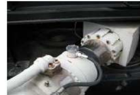
Fig. 11: Magneto Resistive Position Sensor on Rod End Gland
